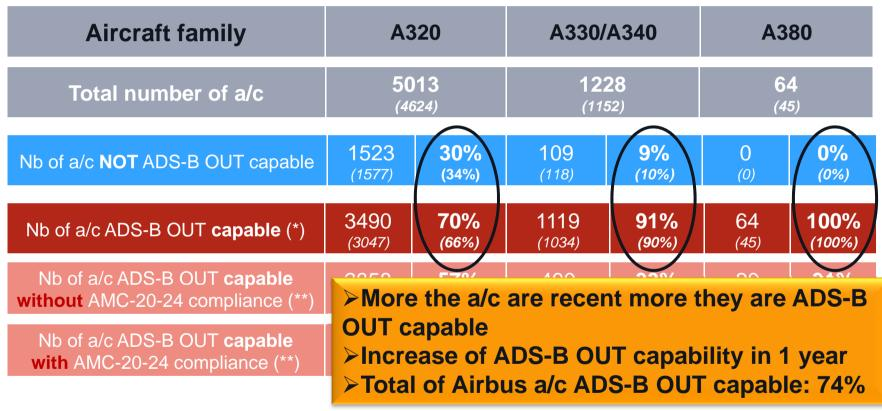
(\*) ADS-B OUT capable means the aircraft is equiped with the required equipments (transponder, MMR...) (\*\*) the AMC-20-24 compliance has to be requested by airline to Airbus (AFM, FCOM update...)
